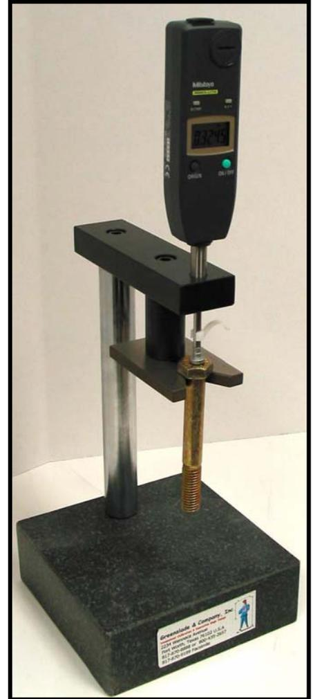
If the user is only interested in measuring head heights this is the gage to select. The "V" arm has an elongated hole so the "V" can be moved toward the back of the gage when measuring large screws and can be moved forward for measuring smaller screws.
